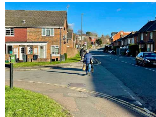
Figure 102. Wide side roads and lack of tactile information and appropriate dropped kerbs reduce the comfort for pedestrians along Upper High Street.
